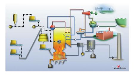
Using Vølund™ technology, B&W's natural circulation boiler fires waste wood (mainly consisting of sawdust, shavings, slip and wood chips) as well as oil and biogas.
